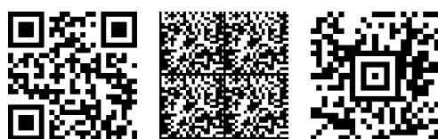
Three common 2D codes in logistics (l-r): QR, Data Matrix, Aztec
